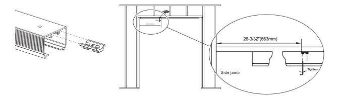
(C) Insert Ball Bearing Hanger Wheel assembly into Track, leave untightened as this will be done latter.
