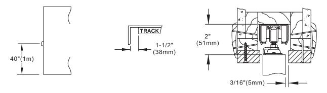
Place the 1st soft close actuator/trigger into the track and have it 26-3/32"(663mm) far from the edge of the side jamb(close to pocket opening). Tighten it to the track.
