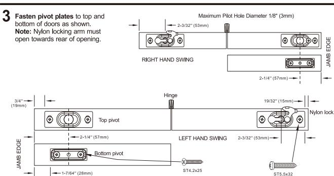
**Fasten bottom pivot bracket** to floor 5/8" (16mm) from jamb face and 7/8" (22mm) from jamb edge. Remove floor bracket and proceed to step 5.
