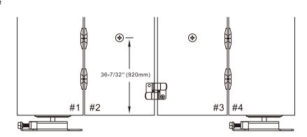
Adjust snubber (track stop) close doors, slide track stop until it touches three-wheeled ball-bearing hanger. open doors, move track stop 1/8" (3mm) closer to three-wheeled ball-bearing hanger and tighten.
